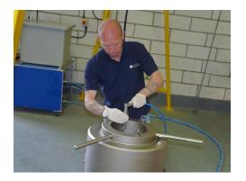
The 6000 metre rated pressure testing facility which is available to hire. Newly constructed in 2009, the chamber has an internal diameter of 340mm with a useable length of 1500mm. These dimensions allow for most transducer assemblies and many towfish designs to be catered for.
